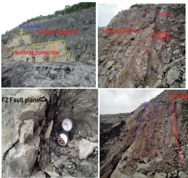
Fig. 3: Shows fault plane condition in the disturbed area
