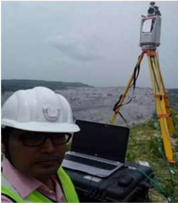
Fig. 6: Lidar laser scanning survey towards south side highwall benches
