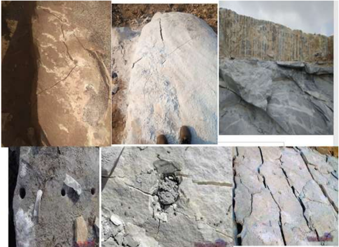
Figure 8 : Shows use of Chemical demolition of oversize boulders and breaking granite blocks in the granite quarry.
